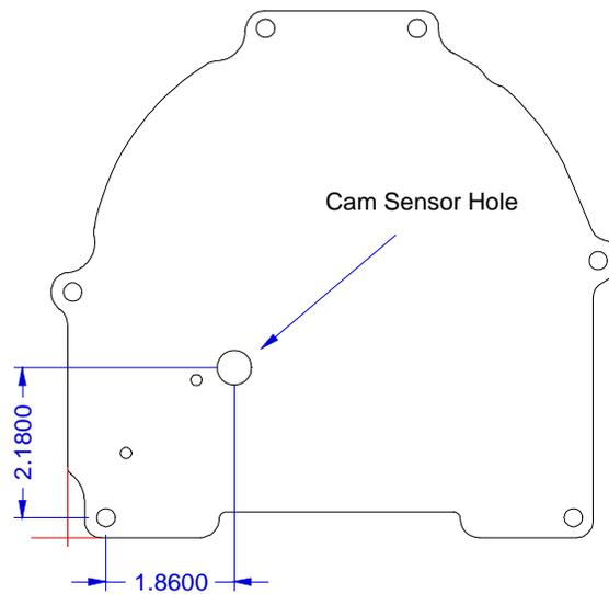
Normally a 15/32" or 1/2" hole will be required for the sensor.
