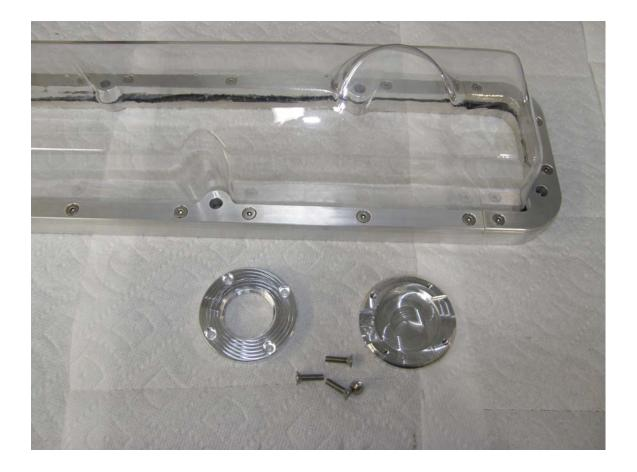
The kit includes the top ring which goes on the outside of the valve cover, the baffle plate which goes on the inside of the valve cover, and four flat head screws. The oil cap, not shown, is also included.
