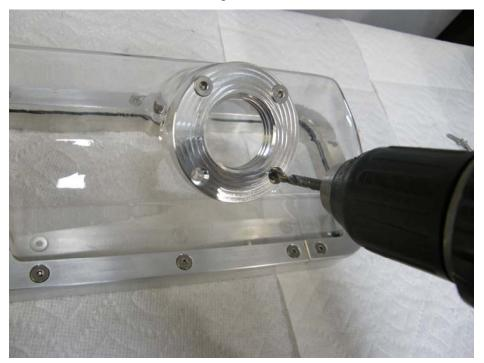
Position all four screws through the top ring. Using your marker or Sharpie again, draw a circle around the inside of the top ring. This material will be cut out of the clear valve cover.
