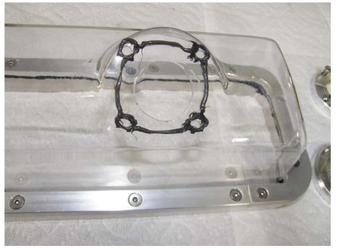
Put the four screws through the top ring and carefully put the ring into place. Reach underneath to install the baffle plate. Look through the clear cover to line the holes in the baffle plate up with the screws from the top ring, and install all four screws loosely.
