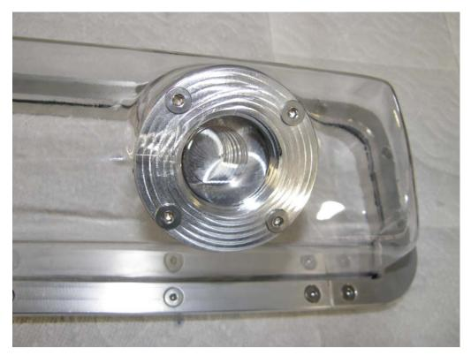
The picture below shows the oil cap assembly with a cap installed; this cap has been fitted with a PCV valve.
