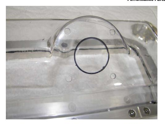
Remove the top ring and screws. Using a step drill positioned in about the center of the marked hole, drill through the clear valve cover. Drill carefully and don't push too hard on the drill; let the step drill do the work.
