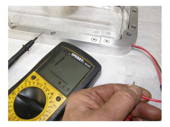
When finished, test to make sure that the LEDs light up. The red wire goes to battery +, 12 volts, and the brown wire goes to battery -, or ground. Hooking the wires up backwards will damage the LED string, so make certain that you connect the wires correctly. Once you have confirmed that the LEDs light up, repeat this process with the other valve cover.
