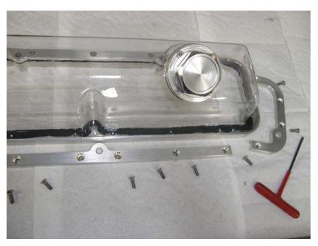
The photo above shows the two aluminum rails removed. Turn the end rail upside down and you will see a slot in the end rail. Remove any burrs of aluminum in this area that may be left over from the machining operations. Position the LED light string so that the wires are in the slot, with most of the black tape out of the slot (there are solder joints under the black tape). The LEDs should be facing in towards the valve cover:
