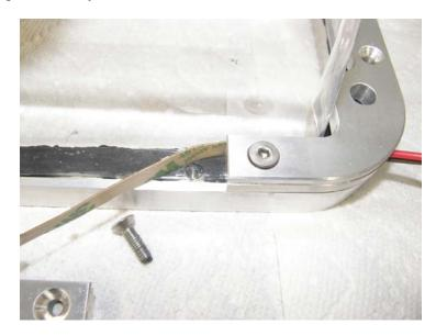
Take the tail end of the LED string and slide it into the gap between the clear valve cover and the other end rail, to hold it in position:
