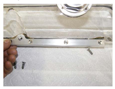
Tighten down all the screws. Check that the end rail is not pinching the wires; the exit of the wires from the end rail should look like this:
