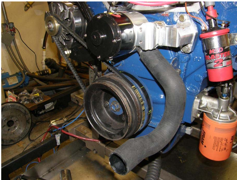
Photo 1 – Modified Dayco 70782 hose installed on CVR Pump
