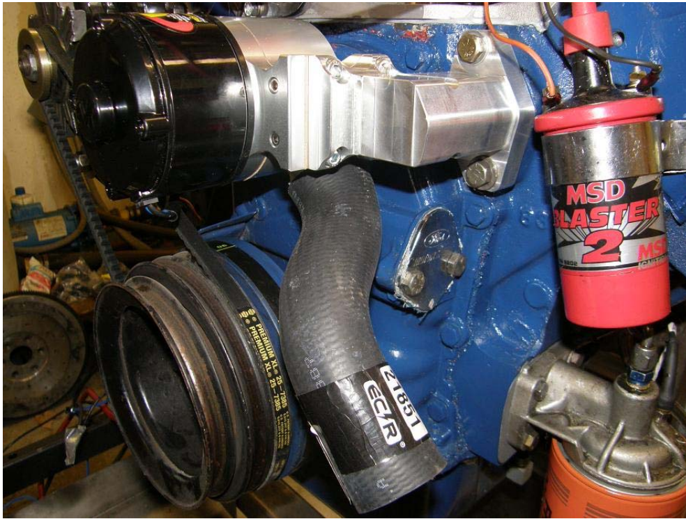
Photo 2 – Modified Gates 21851 hose installed on CVR Pump
