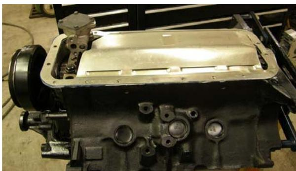
The primary function of the factory windage tray, shown here installed on our engine, is to keep the extra quart of oil in the pan away from the spinning crank. Always run at least six quarts of oil, even in a five quart pan! Mark your dipstick tube accordingly. More info at 428cobrajets.com.
