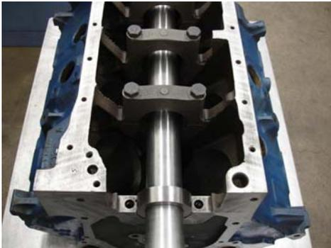
Decking the block starts by bolting this reference bar into the block's main saddle, to provide an index to the crank centerline.
