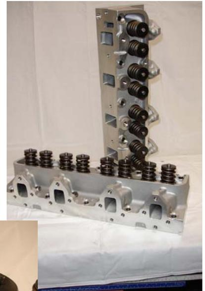
Edelbrock's Performer RPM heads for the FE feature 427 medium riser ports and flow numbers, plus 428 Cobra Jet valve sizes. The heads are available completely assembled, or as bare castings for those who would rather add their own components. For our street motor we started with the assembled set, and then swapped in the 930-16 Comp Cams springs recommended for our cam. The springs were a direct replacement for the Edelbrock springs; even the installed height was correct!
