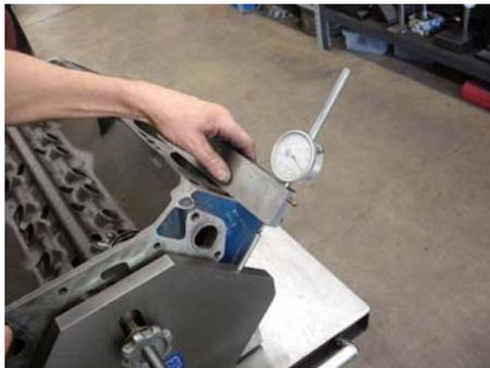
The flat bar with the dial indicator is used to determine the relative block deck heights from side to side. Running the dial indicator along the block deck will give a measurement for how far out of square the deck is with respect to the reference plate. A machinist's straightedge across the decks had shown that they were flat within a thousandth or so, but the dial indicator revealed that the decks were not the same height side to side, and also out of square with the crank centerline.
