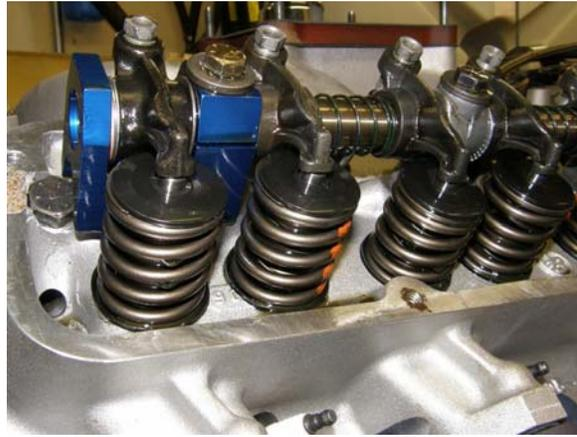
The rocker shaft end stands from Precision Oil Pumps provide support on both sides of the end rocker on each shaft. The factory stands do not provide this support, leading to frequent shaft failures with higher than stock spring pressures. The rockers are the factory adjustable units, and the pushrods are also factory 3/8" ball/cup units. This valvetrain is good to 6500+ RPM with a solid cam and spring pressures up to 400 pounds.
