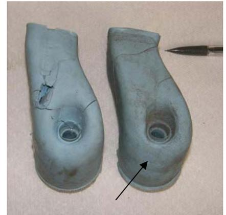
RTV castings were made of the stock Edelbrock intake port, and revealed a necked down area just inside the port entrance (pencil). Also a flat area in the intake bowl was discovered (arrow). The modified port (left) corrects these issues, and leads to improved high lift flow from a two hour home porting effort.
